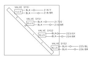
FIGURE 19 - 30, 40 & 50 TON LIQUID LINE SOLENOID WIRING
